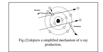
energy of the electron. The vacancy resulting from the ejection is filled by an electron from an outer orbit (e.g. L shell) with lower binding energy, leaving a vacancy in this outer orbit, which in turn is filled by another electron from an orbit even further away (e.g. M shell) from the nucleus.
