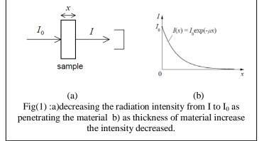
Where I is the transmitted X-ray intensity, I0 is the incident X-ray intensity,  $\mu$  is the linear attenuation coefficient (in cm-1) and x is the thickness of the material (in cm). This equation shows that the X-ray intensity depends on: -The density of the material (the linear attenuation coefficient  $\mu$  increases with density).
